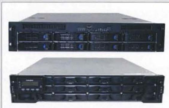
Figure 1: The hardware used for the backup tests, with the ExuS Data server at the top and the transtec RAID at the bottom.
