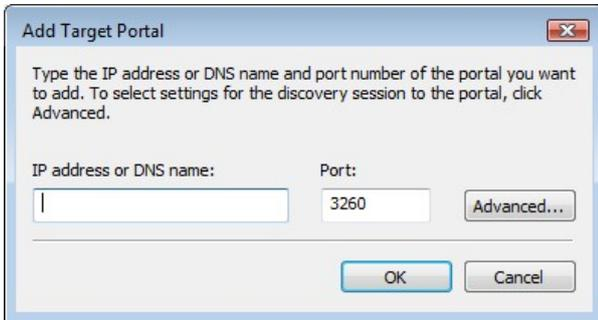
Figure 33 Adding a Target portal
