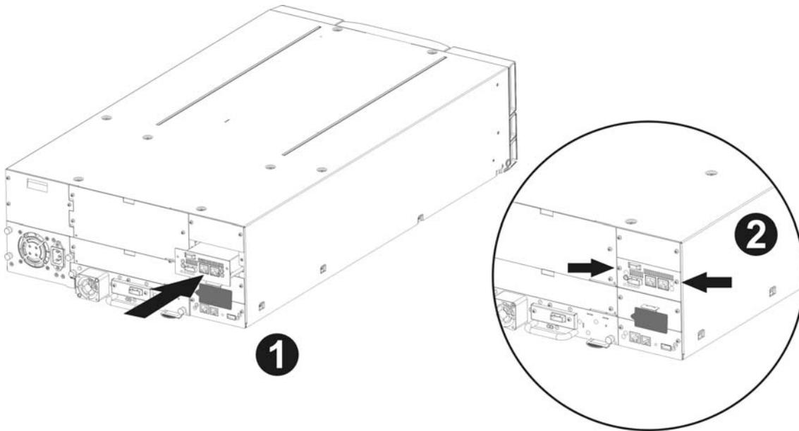
Figure 8 Installing the bridge in the PowerVault TL4000
