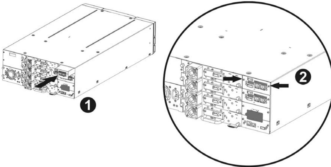
Figure 10 Installing the second bridge in the PowerVault TL4000
